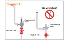
Do not attempt to close a shut-off valve on a meter set that includes a pressure relief valve. Shut-off valves on these meter sets are typically locked and should remain open. (**Dia 1**)
